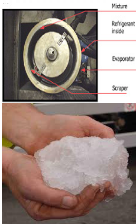
Fig. 2 Mechanical scraped surface ice generator
