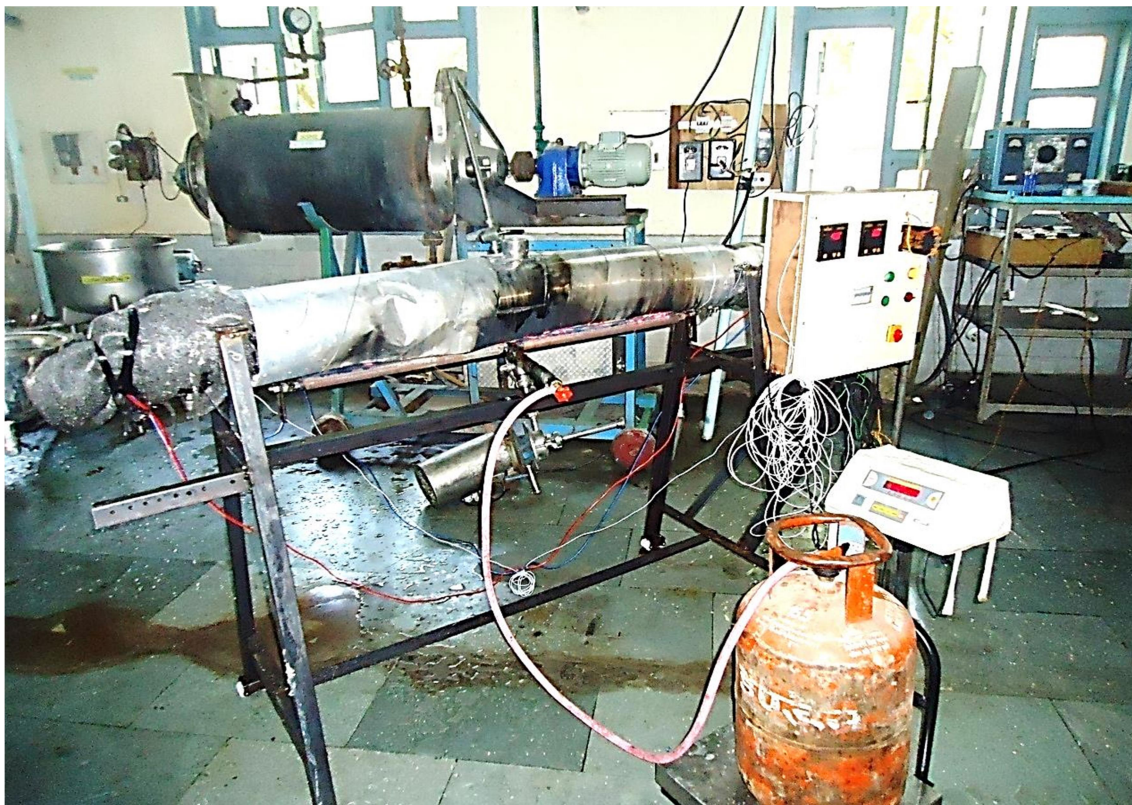
Fig.2: Photograph of developed thermic fluid based heating system
