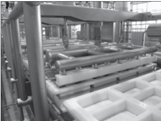
Individual pressing of Paneer in the multimoulds
