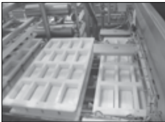
Paneer in multimoulds after Columnar Forming Unit
