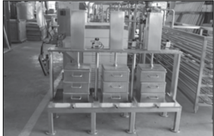
Automatic Paneer Plant, G. K. Dairy : Capacity 1 Ton Per Day
