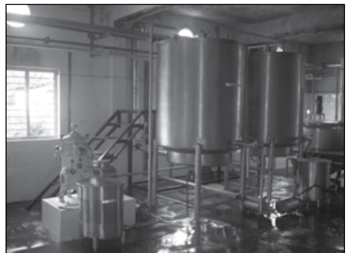
Ghee Plant, Ap Dairy, Karimnagar : Capacity 1 Ton Per Da
