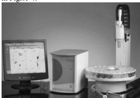
Fig. 1: ASTREE Electronic Tongue Used for taste analysis study and formulation taste assessment, Taste ranking possible
