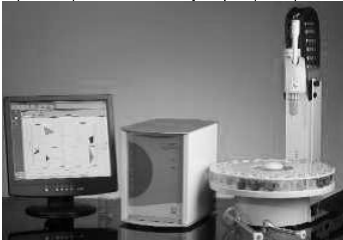
Fig. 5: Astree Electronic tongue system
