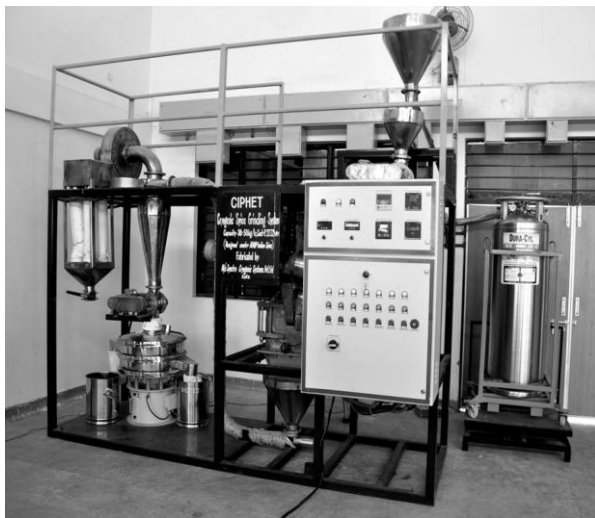
Fig.1: CIPHET – Cryogenic Spice Grinding System
